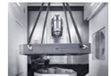
Standard convertible roof facilitating the loading/unloading of pieces by crane.
