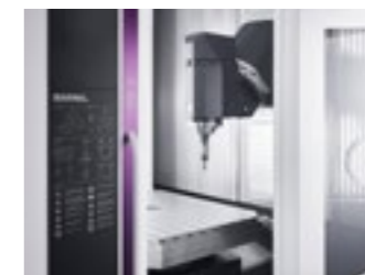
Illuminated working area. Working area without horizontal planes and smooth top.
