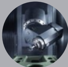
THC_ B axis head Maintain the same tool center point across the full range -15°/+195°
